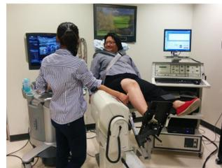
Experimental setup: The participant is seated in a recumbent position that allowed easy monitoring of blood flow with Doppler ultrasound. Force (torque) is measured during muscle contractions using a Biodex dynamometer with an ankle attachment.
