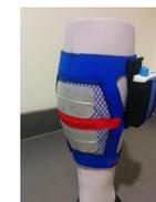
A prototype of the Smart-E-Socks : a garment with integrated electrodes designed to deliver IES to calf muscles.
