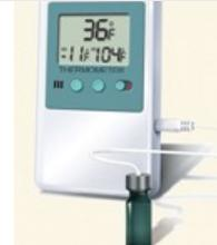
A refrigerator setting of +5.0°C provides the best safety margin for temperature fluctuations within +2.0°C and +8.0°C.
