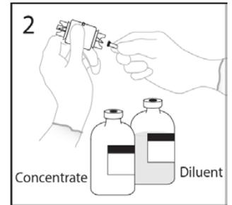
7. Place the diluent vial on a flat surface. Use the exposed end of the transfer device to spike the diluent vial through the centre of the stopper.
