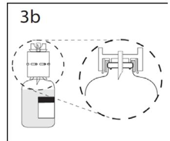
9. Hold the diluent vial with the attached transfer device at an angle to the concentrate vial to prevent spilling the diluent.
